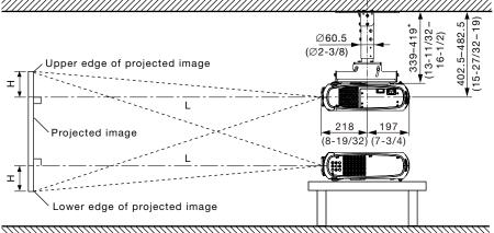
Illustrations show the projector installed using optional ceiling mount bracket ET-PKR100H.
