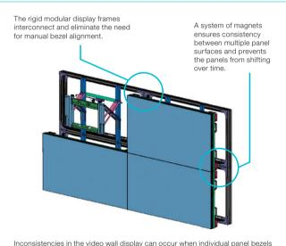
are not correctly aligned vertically and horizontally, and when panel surfaces are not properly adjusted. Surface alignment control magnets and interlocking mounts ensure precision installation in every axis. The Installation Mount facilitates easy setup and makes individual panels easier to remove for maintenance.
